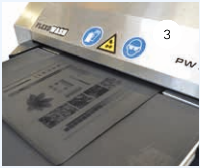
1: Instead of a tray you can add a table for unloading of plates. 2: Sponge roll holder for easy and safe storage of the sponge preventing it from drying out when not used over a longer period of time, 3: With the DLE version you can clean laser engraved plates.
