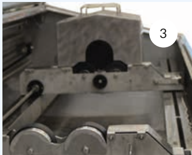
1: For anilox sleeves, an adaptor can be made according to the specific measures of the anilox 2: Recirculation unit for reuse of rinse water, 3: Gear covers for protection of shaft ends.
